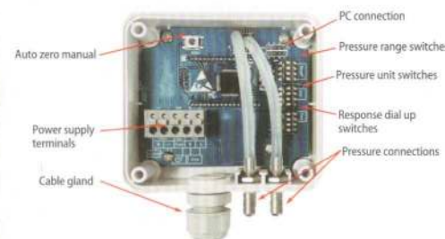
Figure 4 LFM11X-XE(F)X Internal Circuit
